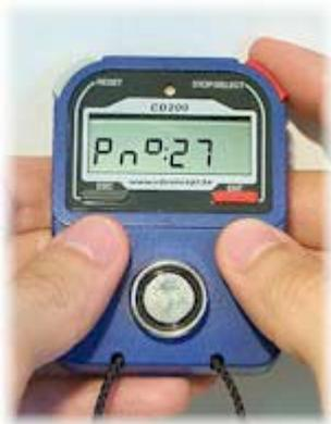
Enter the configuration menu, select 'P n°' function and press the 'ENT' button.
