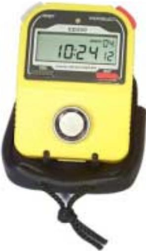
The Rally Timer is a microcomputer mounted inside a stopwatch body which is fitted with an ibutton interface.
