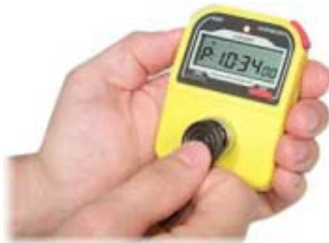
In a fraction of a second, the Start time is recorded into the ibutton and appears on the display for 3 seconds.
