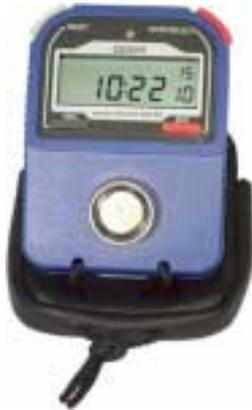
The Rally Manager is a microcomputer mounted inside a stopwatch body which is fitted with an ibutton interface, a serial port and an embedded EEPROM memory.
