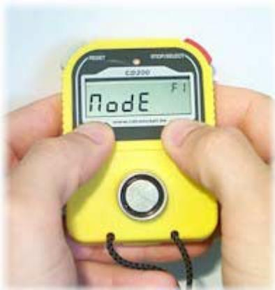
To enter the configuration menu, hold both 'ESC' and 'ENT' buttons for minimum 5 seconds.
