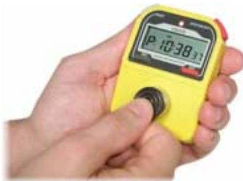
The control worker presents the ibutton to the Rally Timer. In a fraction of a second, the time is recorded into the ibutton and appears on the display for 3 second
